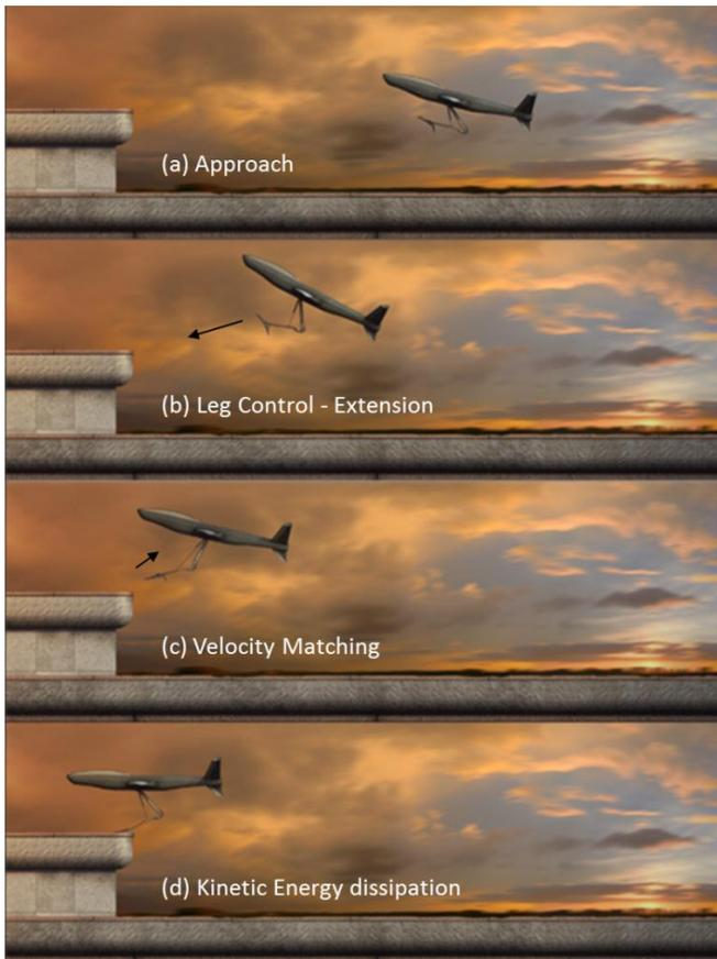
Fig.2. Stages of the perched landing maneuver.
