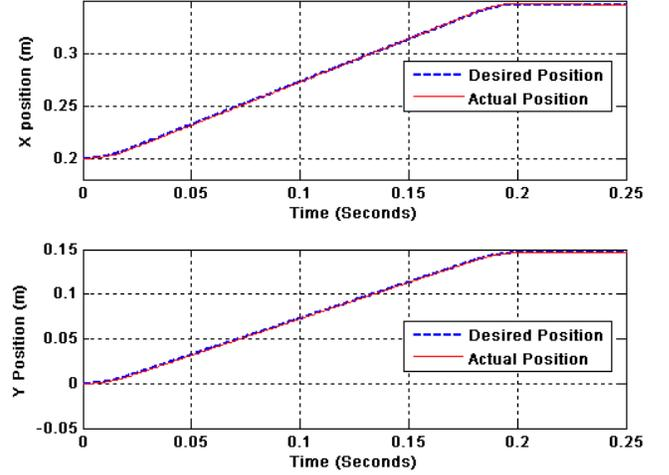
Fig.4. Desired and actual X and Y positions of the end effector during interpolated position control – Computed torque controller with secondary PID controller.
