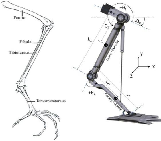
Fig.5. Comparison of the typical anatomy of a bird's leg (left), adapted from the Manual of Ornithology [8] and model of 2-joint mechanical leg (right) showing the centre of gravity of UAVs.
