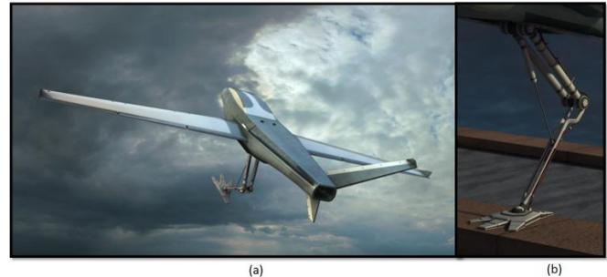
(a) In-flight (b) Close-up view of the landing mechanism.
