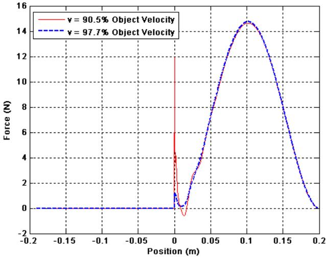
Fig.7. Force experienced during the combined process of velocity matching (prior to position being 0 m), on impact with the perch (at position 0 m), and while decelerating (next section).
