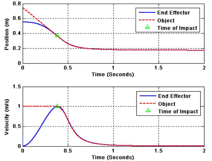
Fig.6. Relative position and velocity graphs of the perch and UAV during the landing maneuver.
