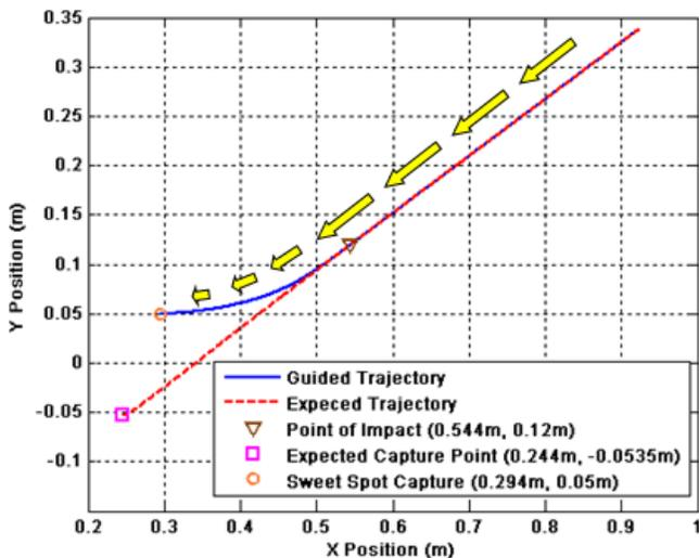
Fig.8. Expected and guided trajectories of the leg during the perched landing maneuver.
