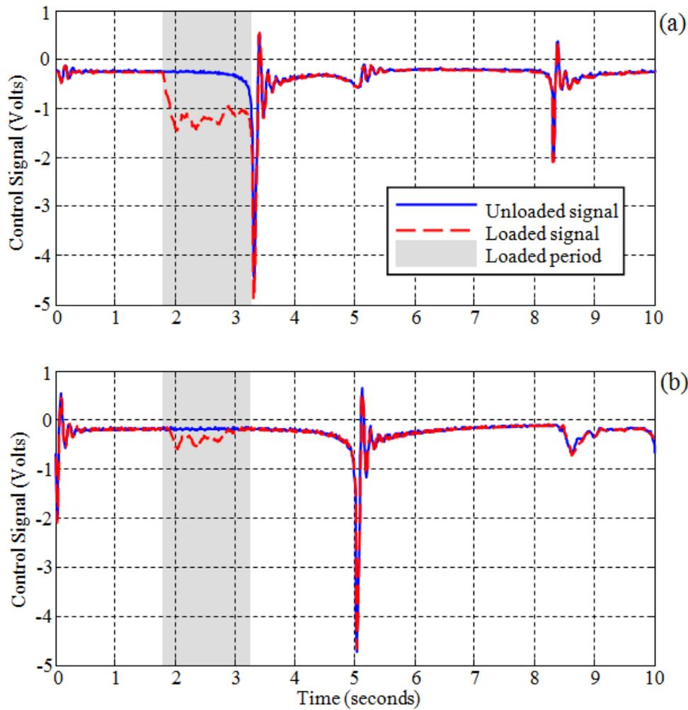
Figure 14: Loaded and unloaded a) upper and b) lower control signals
