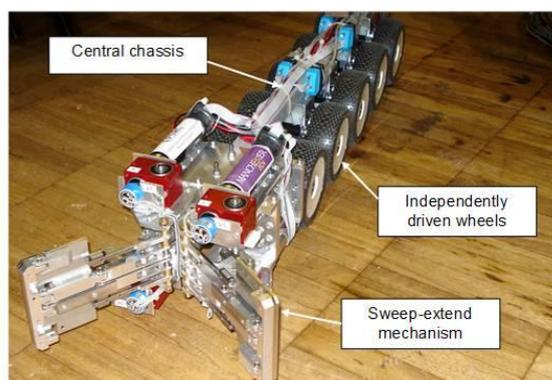
Figure 11: Mechanisms on mobile platform
