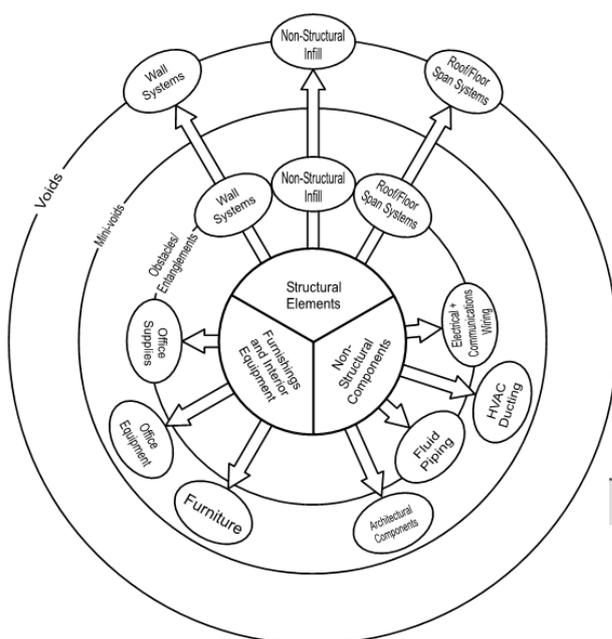
Figure 2 (a): Debris field elements diagram
