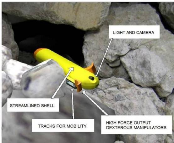
Figure 4: Robot concept
