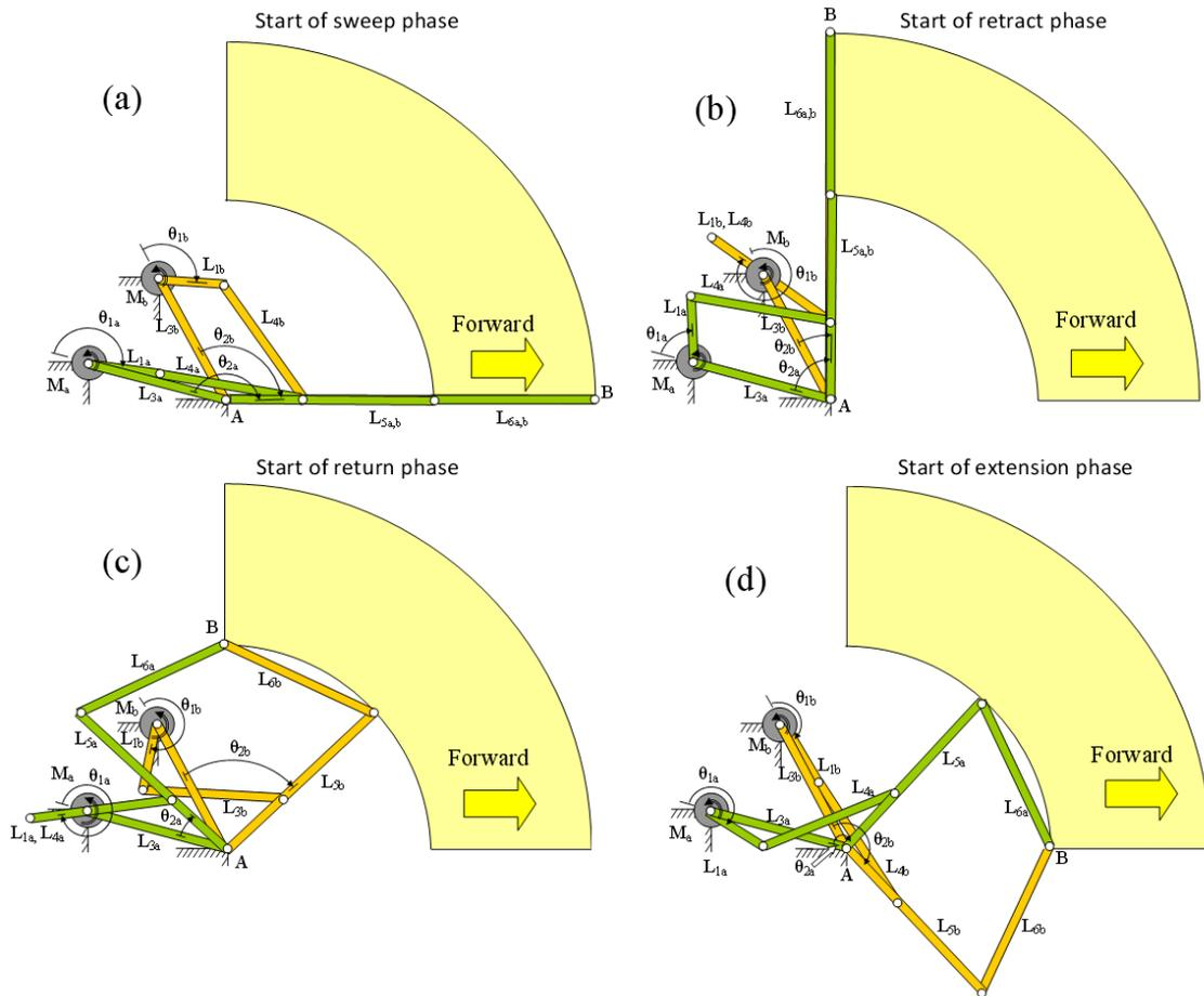
Figure 8: Link positions for workspace key points
