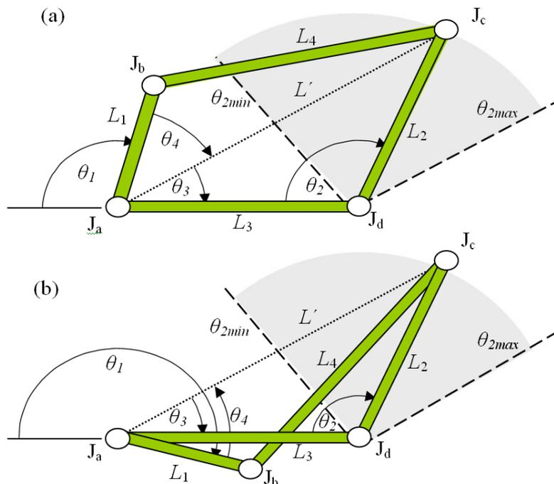
Figure 6: Four-bar mechanism in a) positive and b) negative positions
