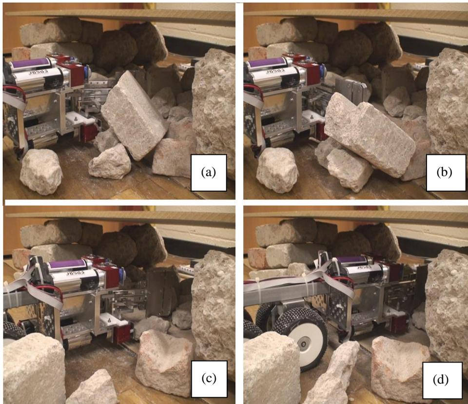
Figure 17: Manipulation of half bricks and concrete
