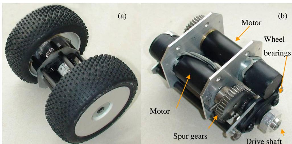
Figure 10: Wheel modules for the mobile robotic base (a) with wheels attached (b) without wheels
