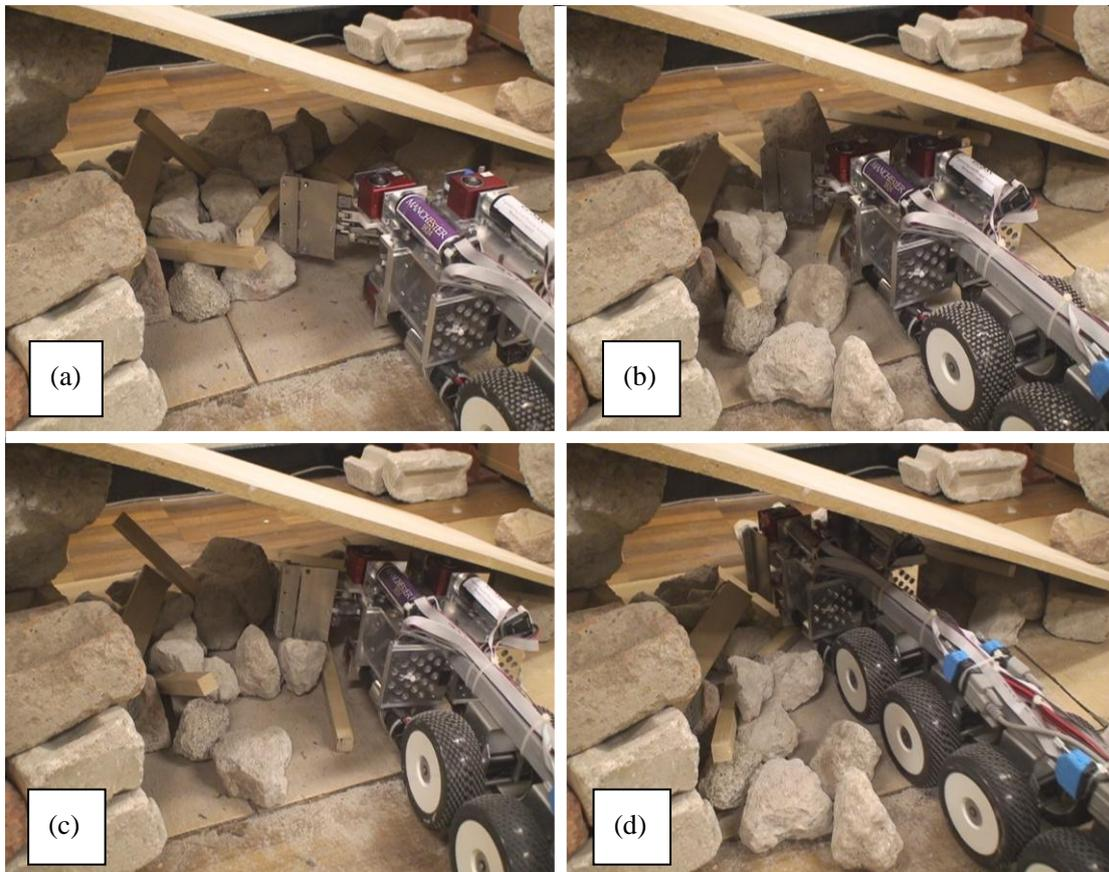
Figure 16: Manipulation of wood and concrete in a lean to collapse
