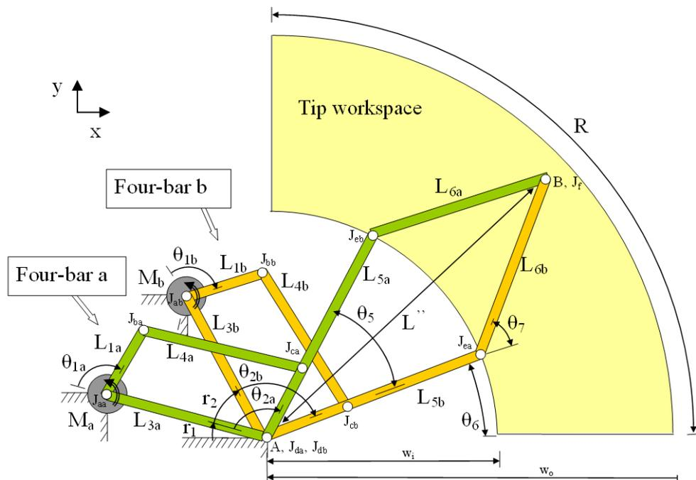
Figure 7: The mechanism configuration and parameters
