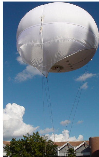
Figure 1. The 13' Kingfisher Aerostat helium balloon.
