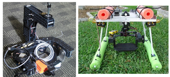
Figure 2. The payload platforms—non-gyroscope-stabilized (left) and gyroscope-stabilized (right).
